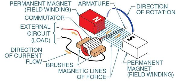
A generator is a device that convert Mechanical energy into electrical energy using electromagnetic induction.
